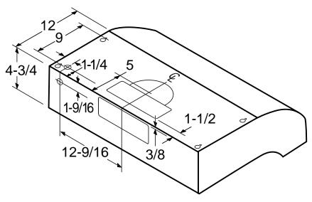
Exhaust outlet connects to 3-1/4" x 10" duct (vertically or horizontally) and 7" round (vertically). Includes rectangular damper and 7" round damper adapter,
