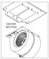
3 Install each blower on the bracket using four nuts per blower.
