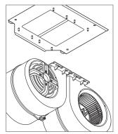
4 Align the tabs on the back of the bracket with the notches at the back of the discharge, then rotate the front of the assembly upward and secure the assembly with the two existing nuts.
