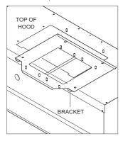
2 For single blowers only, remove the center section from the bracket.
