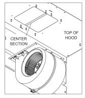
2 Install each blower using four nuts per blower.
