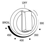
The oven burner should light in 20-40 seconds; this delay is normal. The oven valve requires a certain time before it will open and allow gas to flow. The oven burner will burn until oven temperature has reached 350°F (175°C). After 20-40 seconds, the oven burner will begin to cycle on and off to maintain the 350°F (175°C) temperature.
