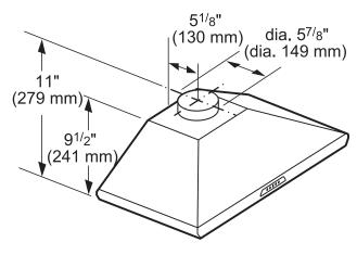
measurements in inches and mm
