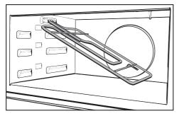
Carefully lower the Browning / Broiling element. The mica sheet can be damaged on the top of the oven cavity. To clean the mica plate, do not use the hard side of the dish-washing sponge.
