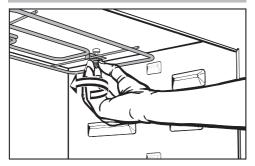
Unscrew the nut and lower the Browning / Broiling element.
