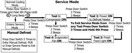
on 1st start-up or power cycle, the compressor will come on after 12 seconds and run 115 seconds. If the door switch is not cycled during this time, the compressor will cut after 115 seconds and not turn back on for another 5 minutes. It may take up to 10 nutes for the compressor to turn on and run in normal mode.
