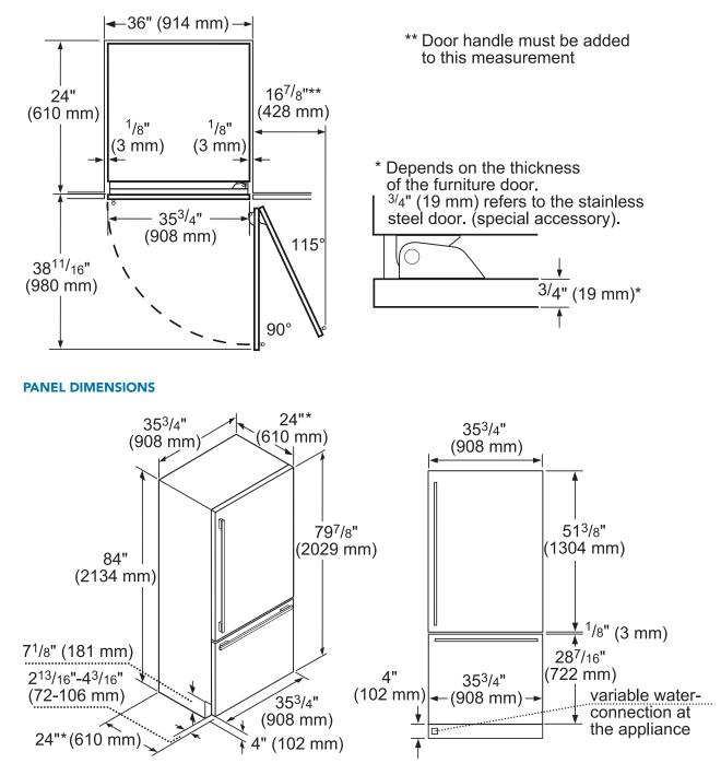
\*Excludes thickness of door panel. If standard panel with <sup>3</sup>/4" thickness is mounted, total depth is 24 <sup>3</sup>/4".
