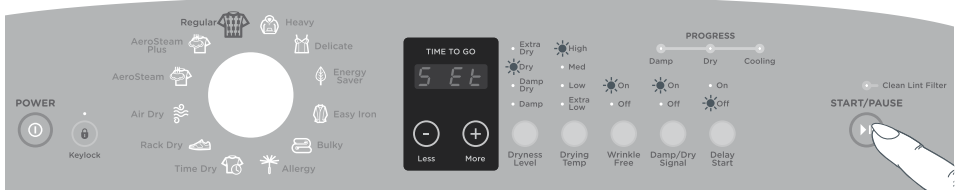
Fig.54 Customizing a drying cycle, eg customizing the WRINKLE FREE option to operate for every REGULAR cycle
