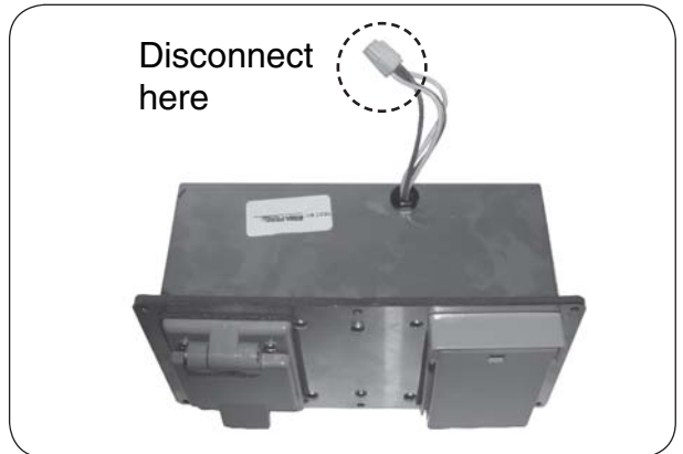
Fig. 32-2 Slightly pull out box and disconnect wire harness
