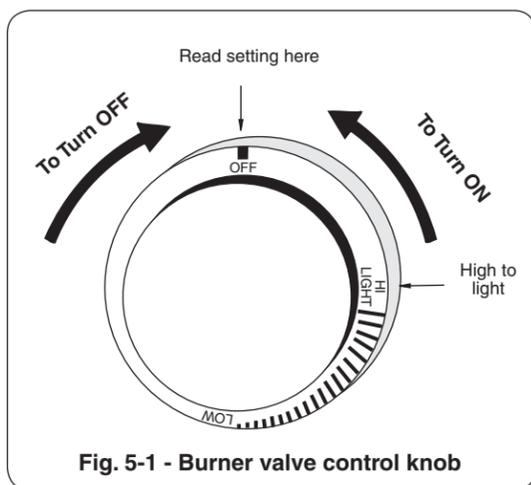
Fig. 5-1 - Burner valve control knob
