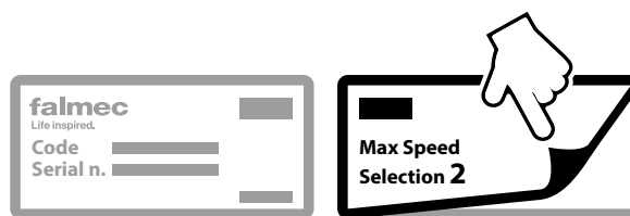
Fig. 2: Set maximum speed 2:
