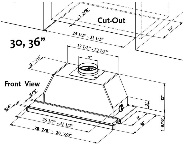
Note: The Cristal comes standard in the top vent position. The direct rear vent position can be achieved by rotating the blower housing.
