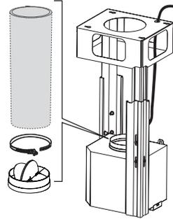
Install Damper that is included with the Hood before connecting to the ductwork.
