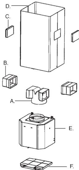
Ductless installations require a **Ductless Conversion Kit** whose components are pictured in **FIGURE 12**. Do not use the DAMPER for ductless installations. The LOWER CHIMNEY COVER should be discarded and replaced by the new one with holes from the **Ductless Conversion Kit (D in FIGURE 12)**.
