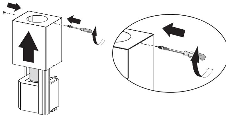
Position the upper chimney section and fix the upper part to the frame using the 2 screws removed previously.
