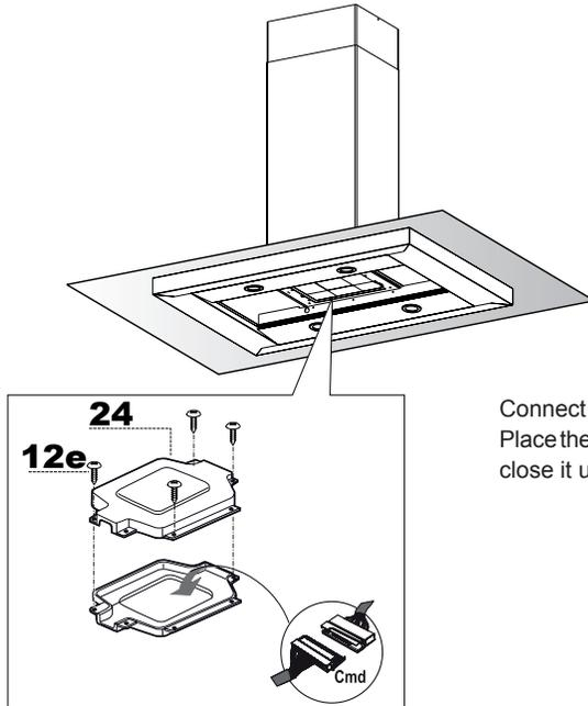
Connect the control connector Cmd.
