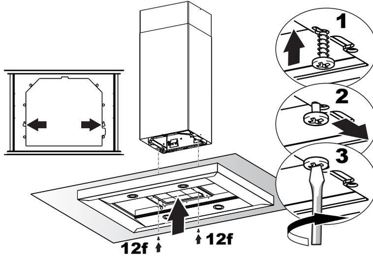
Screw the 2 screws 12f half way into the holes provided in the sides of the bottom of the frame.
