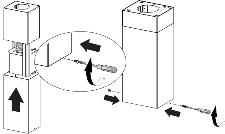
Similarly, position the lower chimney section and fix the lower part to the frame using the 2 screws removed previously.
