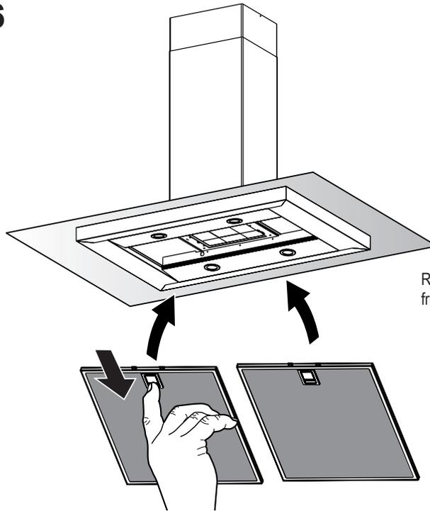
Reinstall the grease filters from the hood canopy.
