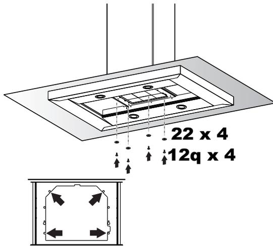
Working from below, fix the hood canopy to the frame where indicated, using the 4 screws 12q and 4 washers 22 provided, then tighten all the screws securely.
