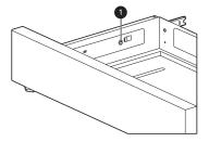
**3** Locate the glide lever on each side of the drawer. Push down on the left glide lever and pull up on the right glide lever.
