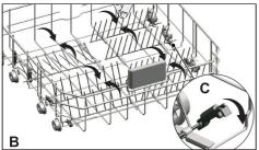
i Bringing the tines to the horizontal position by holding them from the tips may cause them to bend. Therefore, it will be appropriate to bring the tines in the middle to horizontal or vertical position by holding them from their stems and pushing in the direction of arrow.
