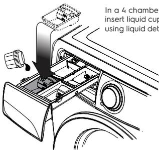
In a 4 chamber dispenser remove liquid cup when using powder detergent! DO NOT pour powder detergent into liquid cup. It will not dispense correctly!
