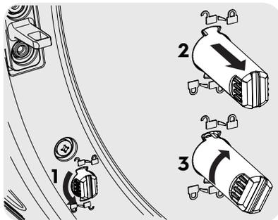
To disengage the stand, rotate to unlock, push the stand in and rotate to lock position.
