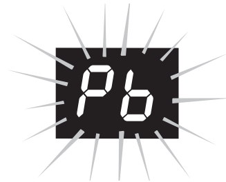
Figure 4: Pb flashes when pan is not making contact
