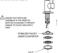
4. SCREW SPRAY HOSE TO THE COPPER PIN (THE LONGEST PIN). MAKE SURE TO HAVE A TIGHT SEAL USING ADJUSTABLE WRENCH. ATTACH SUPPLIED COUNTERWEIGHT TO THE HOSE.
