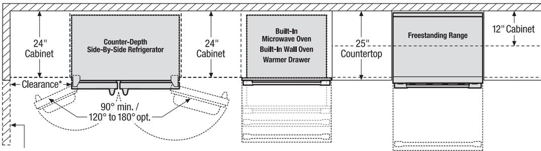
\*When installing side-by-side refrigerator adjacent to wall, cabinet or another appliance that extends beyond front edge of unit, 20" minimum clearance recommended to allow for optimum 120° to 180° door swing, providing complete drawer / crispener access and removal. (Absolute 4-1/2" minimum clearance will ONLY allow for 90° door swing which will provide limited drawer/crisper access with restricted removal.)
