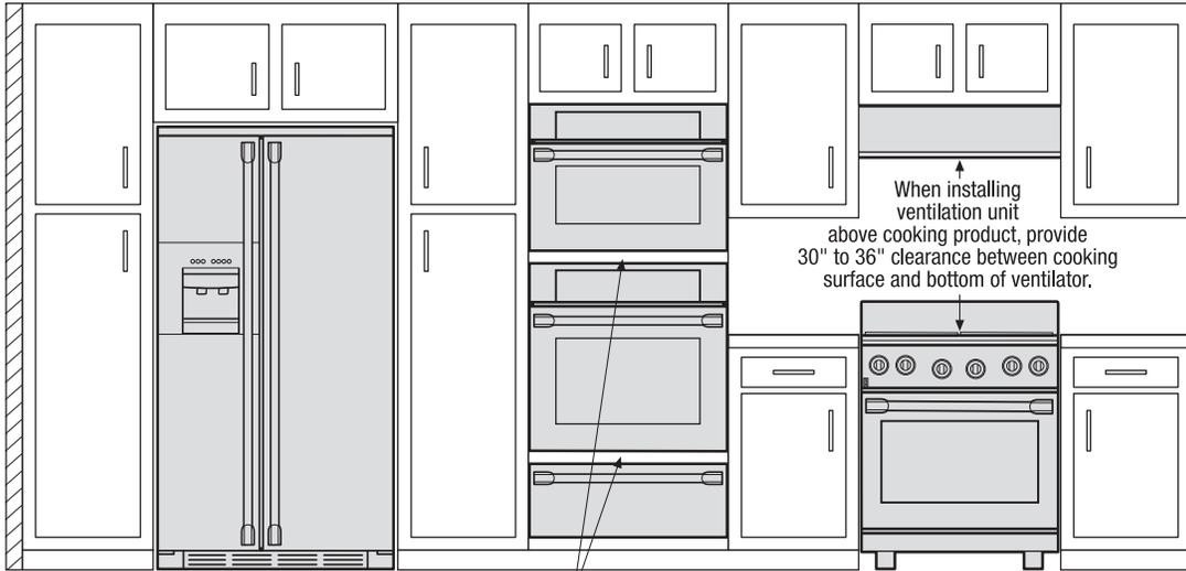
When installing built-in cooking appliances in combination, 2"-high minimum visible gap between appliance faceplates required.
