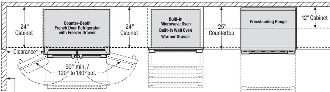
\*When installing French door refrigerator adjacent to wall, cabinet or another appliance that extends beyond front edge of unit, 20" minimum clearance recommended to allow for optimum 120° to 180° door swing, providing complete drawer/crisper access and removal. (Absolute 4-1/2" minimum clearance will ONLY allow for 90° door swing which will provide limited drawer/crisper access with restricted removal.)
