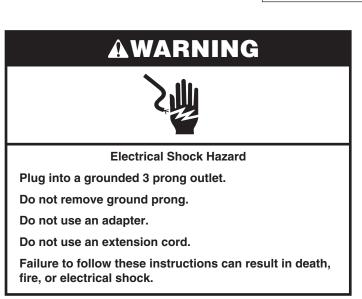
**Electrical:** A 115 V, 60 Hz., AC only, 15 A or 20 A fused, grounded electrical supply is required. It is recommended that a separate circuit serving only your freezer be provided. Use an outlet that cannot be turned off by a switch. Do not use an extension cord.
