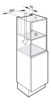
To ensure that the Combi Steam Oven has adequate ventilation, the following cut-outs measuring 19 11/16"  $\times$  1 9/16" (500  $\times$  40 mm) must be made:
