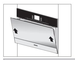
Do not lift the door at the door handle. The handle and door panels could be damaged.
