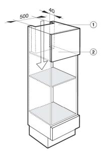
To ensure that the Combi Steam Oven has adequate ventilation, the following cut-outs measuring 19 11/16" x 1 9/16" (500 x 40 mm) must be made:
