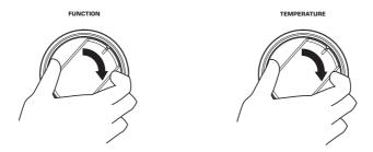
Select the oven function and temperature. Preheat the oven if appropriate. Remember ROAST and CONV BROIL do not require preheating.
