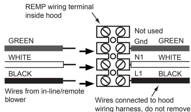
2. Connect the pre-wired, white and green wires to the corresponding black, white and ground (green) wire from the power source wiring. Use wire nut connectors to secure the connections.
