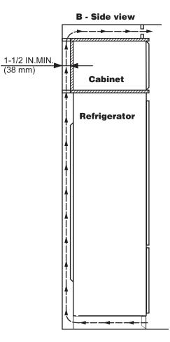
The refrigerator is designed to allow proper air flow when the appliance is installed up against the wall.
