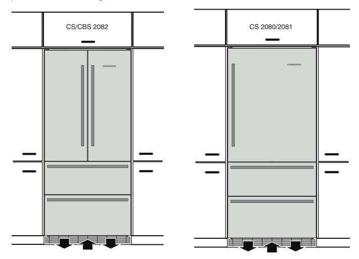
The cover grill provided with the appliance must be used for the ventilation opening. This grill must not be covered by toe kick or other trim.
