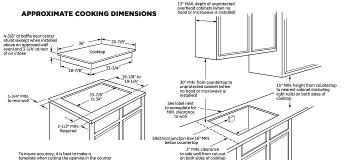
template when cutting the opening in the counter
