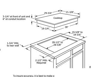
template when cutting the opening in the counter
