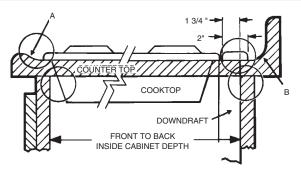
Refer to the cooktop installation instructions for dimensions of cooktop, countertop cut-out, and cabinet requirements. The 2730 and 2736 can be installed in most standard 30" and 36" wide cabinets.
