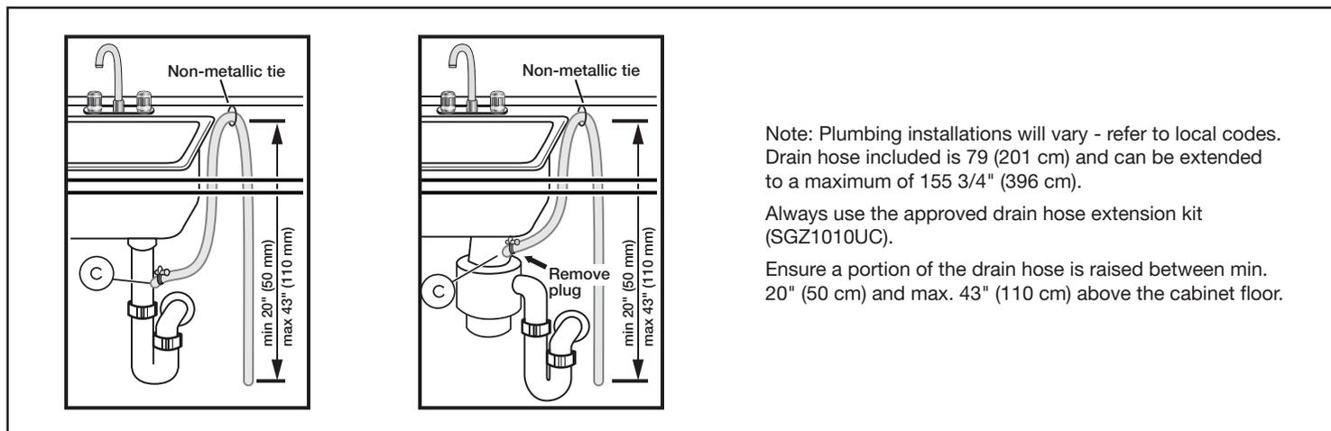
Note: Plumbing installations will vary - refer to local codes. Drain hose included is 79 (201 cm) and can be extended to a maximum of 155 3/4" (396 cm).
