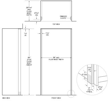
\*3" (76) typical depth. Shaded areas will be visible and should be finished to match cabinetry. NOTE: Shaded line represents profile of unit with <sup>3</sup>/<sub>4</sub>" (19) panel.
