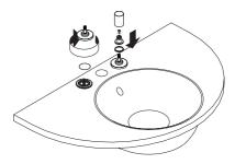
Seat the spout assembly with sealing ring on top of the mounting surface.
