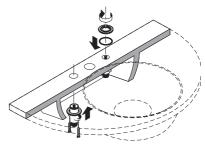
Pull downward on the valve until the mounting ring is seated firmly on the countertop. -Tighten the tensioning screws.
