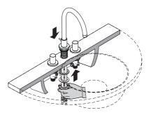
Make sure that the spout assembly stands straight. Tighten the tensioning screws.
