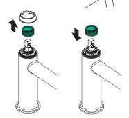
• Reinstall the high temperature limit stop ring so that the black positioning pin is in the notch corresponding to the desired high temperature. The temperatures shown in the diagram assume an incoming cold water temperature of 50°F and an incoming hot water temperature of 140°.
