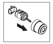
Install the cup washers and springs in the rough. Install the cartridge assembly.
