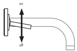
Pivot the handle up to turn the water on, down to turn it off.
