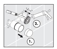
Use a 17 mm socket wrench to remove the spout plug.
