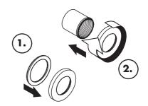
Push the sleeve / handle escutcheon assembly into place over the handle (1). Tighten it by rotating it clockwise (2).
