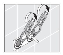
Lightly lubricate the o-rings on the spout and handle escutcheons with the enclosed lubricant (1). Push the escutcheons onto the baseplate.
