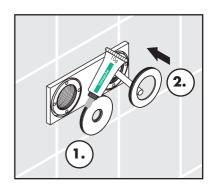
Wrap the threads on the spout with Teflon tape (1). Install the spout (2). Install the handle flange (3).
