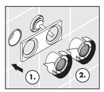
Tighten the retaining nuts with the service key.
