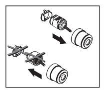
Install the new cup washers and springs in the rough. Install the cartridge assembly.
