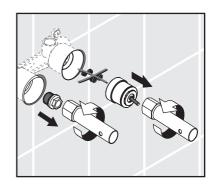
Remove and discard the cartridge and anti-twist device from the housing. Install the new cartridge and anti-twist device in the housing.
