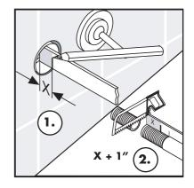
Install the spout escutcheon on the spout. Push the sealing ring into the spout escutcheon.
