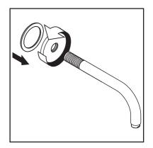
Wrap the threads on the spout with Teflon tape (1). Install the spout (2).
