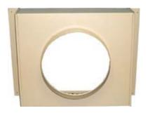
EP ... Evaporator Return Plenum attaches in place of the standard return air grille allowing a ducted return. Great for remote cooling of computer and equipment rooms. 10 inch round duct for the PWC10 and 12. 12 inch round duct for the PWC18, 24. And, 16 inch on the PWC36 and PWC60
