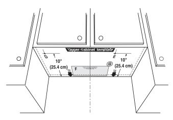
5. Cut the 11/2" (3.8 cm) diameter hole at the circular shaded area "G" on the template. This hole is for the power supply cord.
