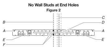
**NOTE:** If wall stud is within 6" (15.2 cm) of the vertical centerline (see "Mark Rear Wall" section), only recirculation or roof venting installation can be done.
