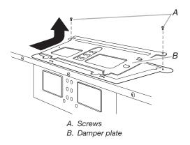
2. Keep damper plate and screws together and set aside.
