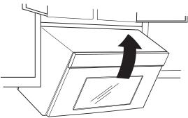
5. Rotate microwave oven up toward upper cabinet. NOTE: If venting through the wall, make sure the damper assembly fits easily into the vent in the wall cutout.
