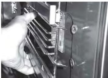
**To remove the oven rack support for cleaning**, support and lift front bottom of rack support to release front tabs. Then rotate rack support up and out to release rear tabs.
