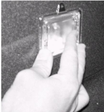
Replace glass shield after replacing bulb
