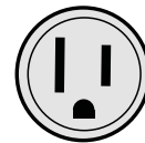
3-pronged Grounding Receptacle 15 Amps. 125V.
