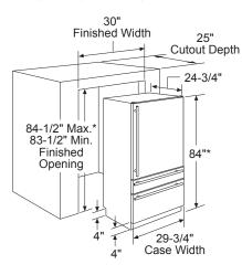
\* 84" High installation. The refrigerator can be adjusted to fit into a cutout that is 83-1/2" min. to 84-1/2" max with the appropriate door kit. Use leveling legs and wheels for a maximum 1" height adjustment.
