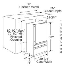
\* 80" High installation. The refrigerator can be adjusted to fit into a cutout that is 79-1/2" min. to 80-1/2" max. height. Use leveling legs and wheels for a maximum 1" height adjustment.
