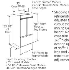
\* Shipping height. The refrigerator can be adjusted to fit into a cutout that is 83-1/2" min. to 84-1/2" max. height. Note that the top case trim at the front is 1/2" higher and will overlap upper cabinetry or soffit. Use leveling legs and wheels for a maximum 1" height adjustment.
