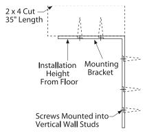
• Secure the bracket with wood block to the back wall so that it is 84" (or your installation height) from the finished floor. Use #12 or #14 wood screws. See illustration.
