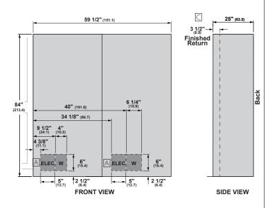
DUAL INSTALLATION 30" INTEGRATED FREEZER, ZIF301NPNII AND 24" INTEGRATED REFRIGERATOR, ZIR241NPNII
