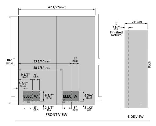
DUAL INSTALLATION 24" INTEGRATED FREEZER, ZIF240NPKII AND 30" INTEGRATED REFRIGERATOR, ZIR300NPKII
