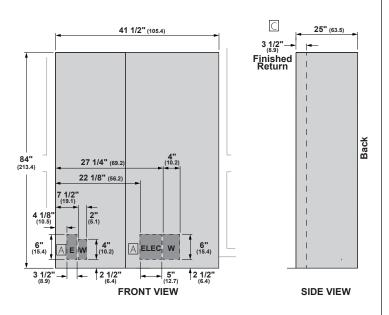
DUAL INSTALLATION 18" INTEGRATED FREEZER, ZIF181NPNII AND 30" INTEGRATED REFRIGERATOR, ZIR301NPNII
