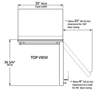
\*\* These refrigerators are equipped with a 2-position door stop. The factory-set 130° door swing can be adjusted to 90° if clearances to adjacent cabinets or walls is restricted. Allow a 15" minimum clearance to wall for pan removal. If the 90° door stop position is used, pan access is maintained, but pan removal is restricted.
