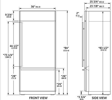
\* Shipping height. Use leveling legs and wheels for maximum 1" height adjustment from shipping height.
