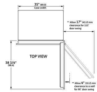
\*\* These refrigerators are equipped with a 2-position door stop. The factory-set 115° door swing can be adjusted to 90° if clearances to adjacent cabinets or walls is restricted. Allow a 15" minimum clearance to wall for pan removal. If the 90° door stop position is used, pan access is maintained, but pan removal is restricted.
