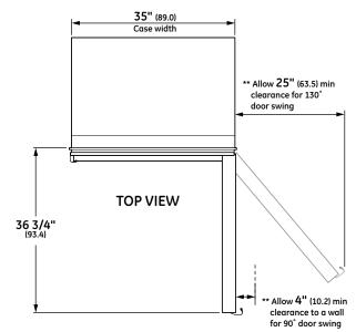
\*\* These refrigerators are equipped with a 2-position door stop. The factory-set 130° door swing can be adjusted to 90° if clearances to adjacent cabinets or walls is restricted. Allow a 15" minimum clearance to wall for pan removal. If the 90° door stop position is used, pan access is maintained, but pan removal is restricted.
