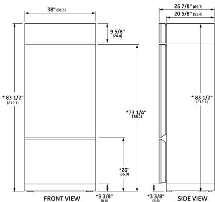
\* Shipping height. Use leveling legs and wheels for maximum 1" height adjustment from shipping height. Nominal installation height is 84"
