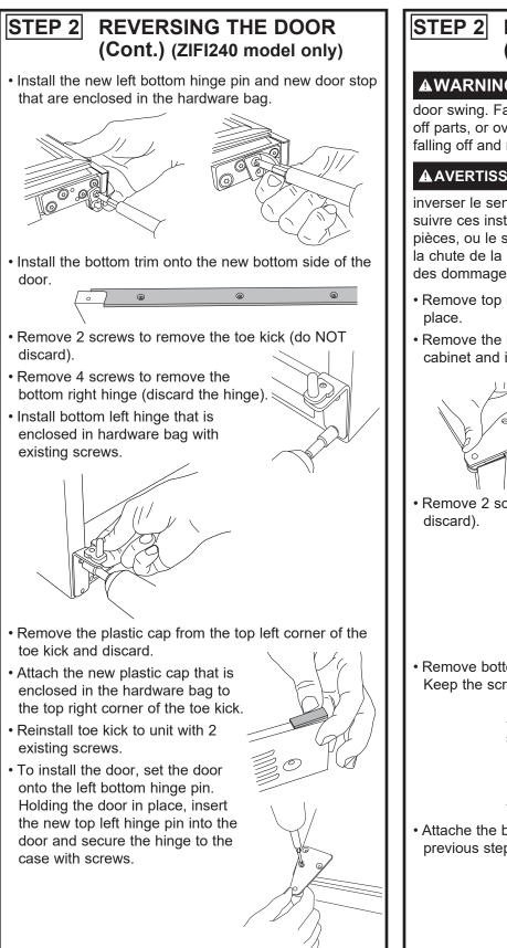
**AWARNING** Follow all steps when reversing the door swing. Failure to follow these instructions, leaving off parts, or overtightening screws, can lead to the door falling off and result in injury and property damage.
