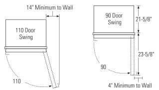
**NOTE:** Clearances are based on the recommended 2-1/4" handle standoff depth.
