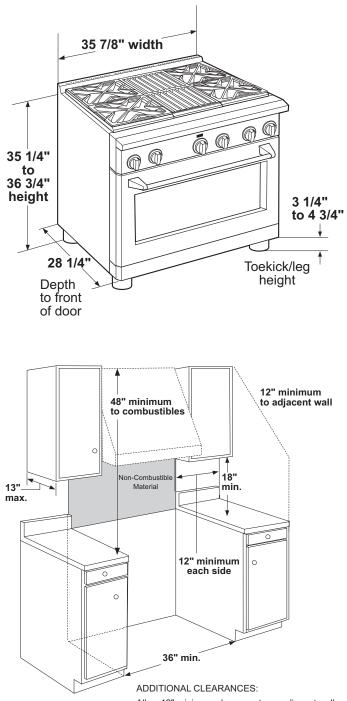
Allow 12" minimum clearance to an adjacent wall on each side.
