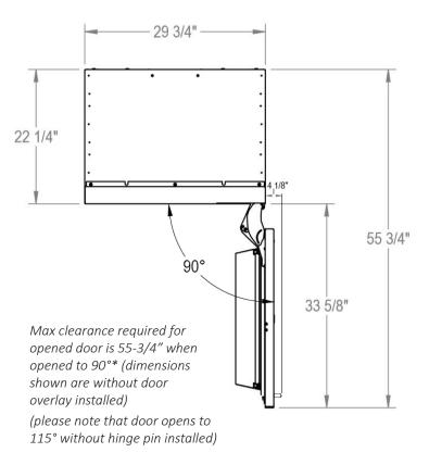
**PLEASE NOTE:** When installing column adjacent to wall, a 2" clearance is required if door opens towards the wall \*90° achieved when included hinge stop pin is installed. Pin must be installed prior to full integration
