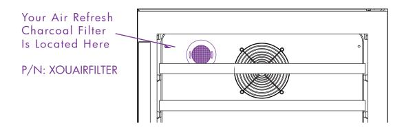
Rotate the filter 1/4 turn to unlock
