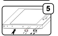
**Step 5:** Reinstall the hardware from the bottom of the door removed in **Step 4** in the holes provided in what had previously been the top of the door.
