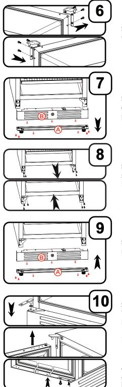
**Step 6:** Remove the upper hinge on the cabinet and replace it with the opposite facing upper hinge, supplied.
